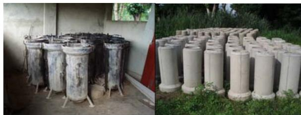
**Figure 7: Moulds (left) and concrete pipe (right) used for the construction of wastewater network in Ewawu area (Kara Togo)**
